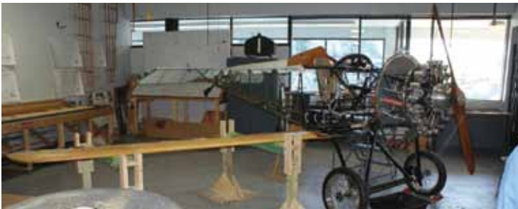
AIM-Chesapeake's Nieuport 24 biplane under construction
